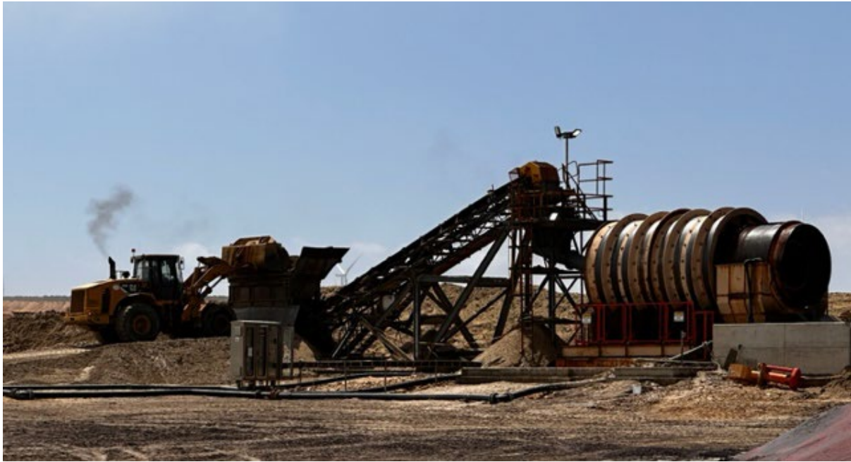
Figure 1 Loading Inland Strands Ore to feed Scrubber to break-up agglomerates and remove slimes
