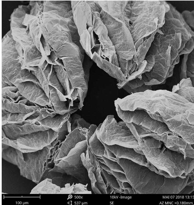
**Figure 2 – SEM micrograph of expanded +180 micron/-300 micron graphite**
