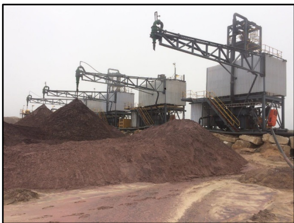
Two Primary Beach Concentrators and the two recently constructed and commissioned Tailing Scavenger Circuits. Depicting Heavy Mineral Concentrate production and stockpile.
