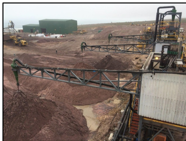
Two Primary Beach Concentrators and the two recently constructed and commissioned Tailing Scavenger Circuits. Depicting Heavy Mineral Concentrate production and stockpile.
